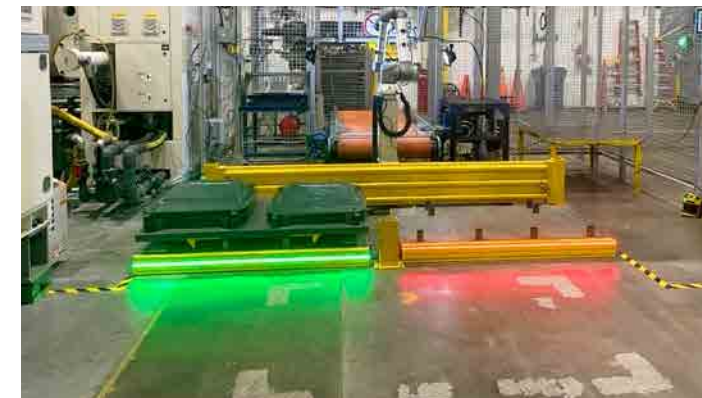
Movement sensors installed to prevent anyone that approaches the cobot area from being hit by cobot.
